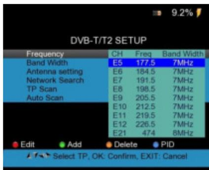
2. **Bandwidth:** Displays the bandwidth of the currently selected transponder.
