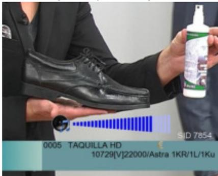
8. **F1 key:** Press the F1-button in the Live TV view and the information field of the current station with information on the signal level and quality is displayed, as well as information of the transponder and transmitter:
