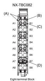
Symbol Name Function The terminal numbers (A1 to A8 and B1 to B8) are displayed. (A) Terminal number indications The terminal number indicators are the same regardless of the number of terminals on the terminal block, as (B) Release holes Insert a flat-blade screwdriver into these holes to connect and remove the wires. (C) Terminal holes The wires are inserted into these holes. (D) Ground terminal mark This mark indicates the ground terminals. Only the NX-TBC082 has this mark.
