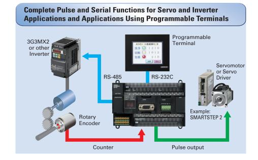
For positioning or communications, simply enter the set values for the instructions. Even complicated functions can be easily programmed using the OMRON Function Block (FB) Library.
